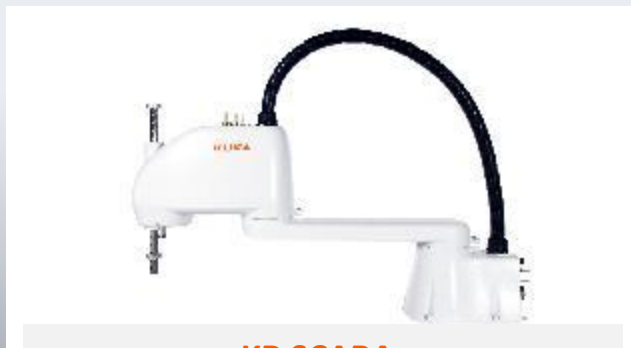
KR SCARA: fast assistants for industrial production
